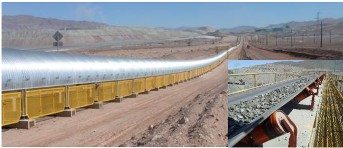
Fig.2 View of a large-scale overland belt conveyor system in service at a large copper mine site.
